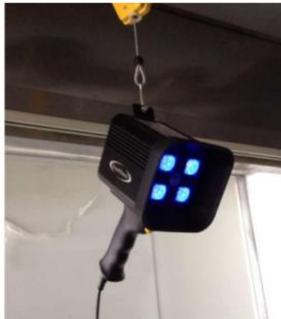
Mounting with spring balance and hook
